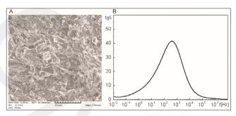
**Figure 2.** A) Scanning electron microscopy image of a fracture of a ceramic matrix (p - 20 MPa,  $T_{cal} = 1100^{\circ}\text{C}$ ); B) Frequency dependence of dielectric absorption of the composite shield at 16°C and relative humidity of 60%
