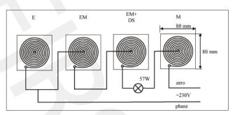
Figure 3. Schematic diagram of equipment used in the application of EMF
